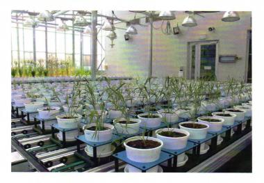
The automated phenotyping system consists of 600 pot carriers on a 250 m conveyer belt system for high-throughput imaging with two cameras, visible and hyperspectral.
